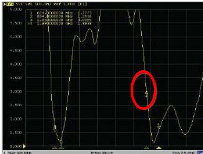
VSWR measured with foil label on
